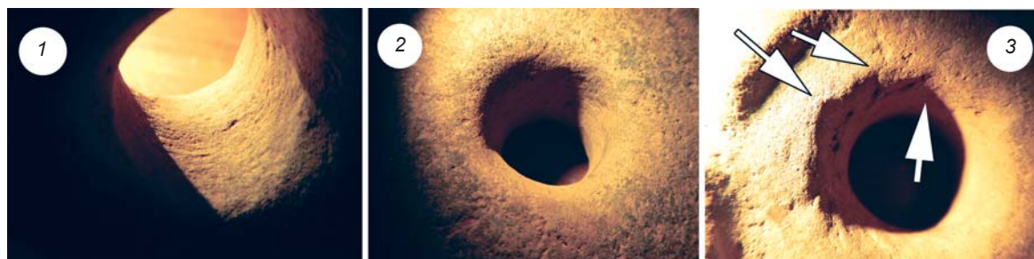
Fig. 4. Surface inside the hole of the disc-shaped item (1), on the entry (2) and exit (3) sections of the drilling channel.
